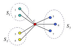
Figure 4. Node C is a partition node. Its neighbor set would be partitioned into three unreachable subsets  $S_1$ ,  $S_2$  and  $S_3$  when C fails.
