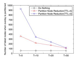
Figure 9. Enhancing resistance to overlay partitioning. It shows the number of failed nodes when overlay is partitioned, with recovery T=5,10,20,50 and TTL=3,4.
