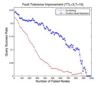
Figure 10. Overlay's fault tolerance improvement. It shows the network's query success rate when nodes continuously fail.
