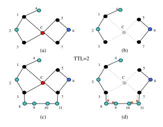
Figure 1. Cut Node vs. Partition Node. (a) C is a cut node because (b) when C fails, the overlay network is partitioned; (c) C is a partition node because (d) when C fails, the overlay network is not partitioned, but C's neighbors 1,3,5,7 can no longer find each other.
